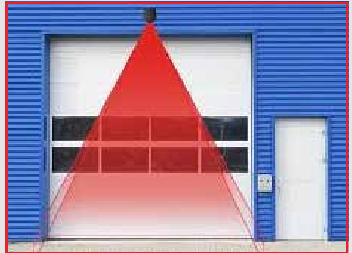
Figure 3.9 Example of a laser scanner installer on an industrial door.
